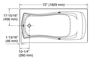
No change in measurements if connected with drain illustrated. (K-7272)
