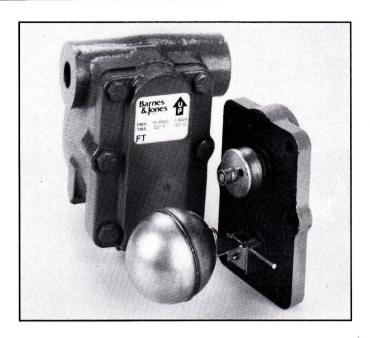
When the water level drops, the weight of the float closes the valve. As condensate enters the traps, the float rises and opens the valve, allowing the condensate to be discharged. The float is designed to provide sufficient buoyancy to overcome the differential pressure across the valve. The internal float and valve configuration is such that the condensate level is always above the valve, creating a continuous water seal at the seat.
