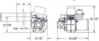
The Air Tube Length (Dimension A) is the distance from the front of the burner housing to the end of the air tube.
