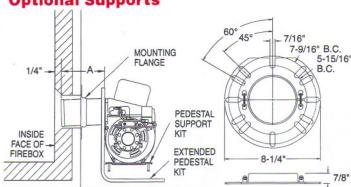
No. 5685 Pedestal Support For conversion applications. No mounting flange is required. Note: Part No. 5606 Extended Pedestal Support is also available, and provides elevation from 8-1/4" to 13". No. 5850 or 5432 Adjustable Mounting Flange Kit
