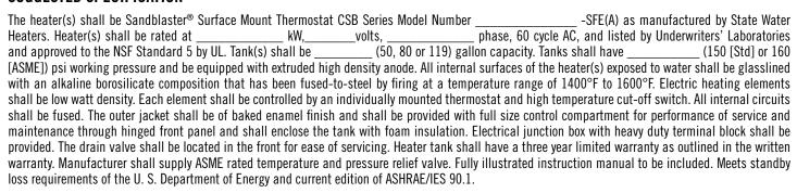
For ASME Construction add "A" to the end of the model number (example: CSB 52 24 SFEA).
