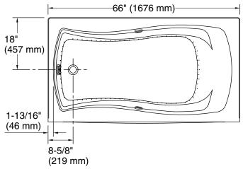
No change in measurements if connected with drain illustrated. (K-7166AF)
