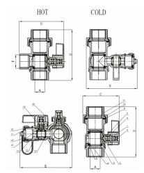
Specifications: Designed for use with water, oil, glycol mix in residential or commercial plumbing and heating systems. Threaded (NPT) ends comply with ANSI B1.20.1. Solder joint temperature ratings are per ASME B16.18 Annex A for 95-5 solder. Do not silver braze or overheat valves when soldering. PEX ends are in accordance with the referenced ASTM specification; refer to tubing manufacturer for installation instructions.
