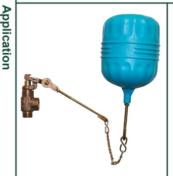
PRIER's 370 Liquid Level Control Valve is designed for cooling towers, stock tanks, poultry troughs, oil level control or any use where liquid level control is desired. The valve is heavy patterned casted brass with a neoprene valve seat. It features positive opening or closing with no leaks or chatter. The 370 Liquid Level Control Valve is available in 1/2" or 3/4" inlets. Each valve is individually tested to assure proper functionality.
