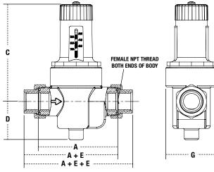
ABOVE VALVE SHOWN WITH SINGLE NPT UNION CONNECTION ON INLET VALVES MAY BE ORDERED WITH 0,1,0R 2 UNION CONNECTIONS USING ANY COMBINATION OF NPT, SOLDER, PEX OR CPVC CONNECTIONS REQUIRED "F" DIMENSIONS ARE APPROXIMATE ENGAGEMENT LENGTHS.
