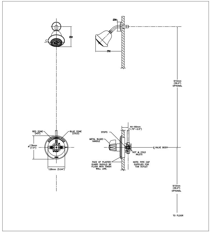
Delta reserves the right (1) to make changes to specifications and materials, and (2) to change or discontinue models, both without notice or obligation. Dimensions are for reference. Measurement may vary plus or minus 6mm(0.25"). Mounting locations are suggested only. Check with local codes for requirements in your area. This spec was produced July 19, 2018.
