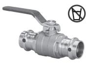
Description Viega ProPress model 2973 is a two-piece. full port ball valve intended for hydronic and nonpotable applications. The ball valve features EPDM sealing elements, EPDM
