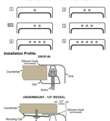
\*Designed to affix to the underside of any solid surface countertop.
