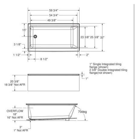
Wood support design may vary, Single Integrated tiling flange: 1" height x 1/4" thickness (shown) All dimensions are approximate. Structure measurements must be verified against the unit to ensure proper fit.
