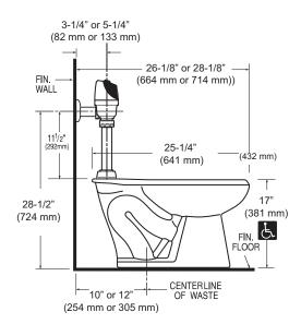
**NOTE**: All vitreous china dimensions shown in these drawings are nominal. Dimensions can vary within the tolerances established in the governing ASME A112.19.2/CSA B45.1 standard. Please take this into consideration when planning rough-in and plumbing layouts.
