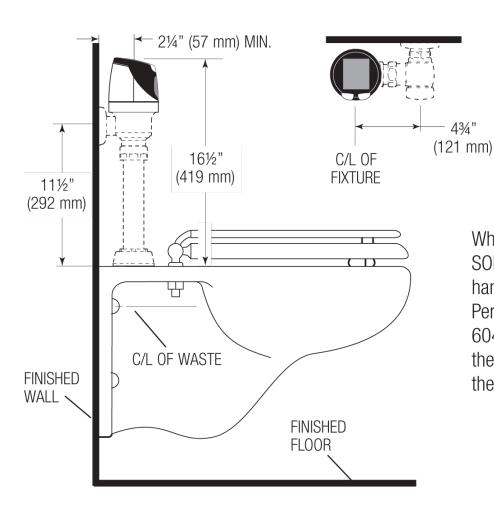
When installing the Sloan SOLIS™ Flushometer in a handicap stall: Per the ADA Guidelines (section 604.9.4) it is recommended that the grab bars be split or shifted to the wide side of the stall.
