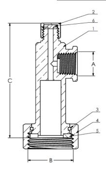
Specifications: Designed for residential, commercial or industrial use with water, oil or gas. Threaded ends comply with ANSI B1.20.1
