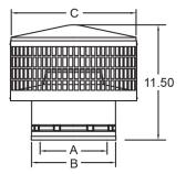
This cap is similar to TGC, but is produced without twist locking buttons. Cap slips onto pipe and is attached with packaged screws. Easily removed for cleaning. See TGC size chart.
