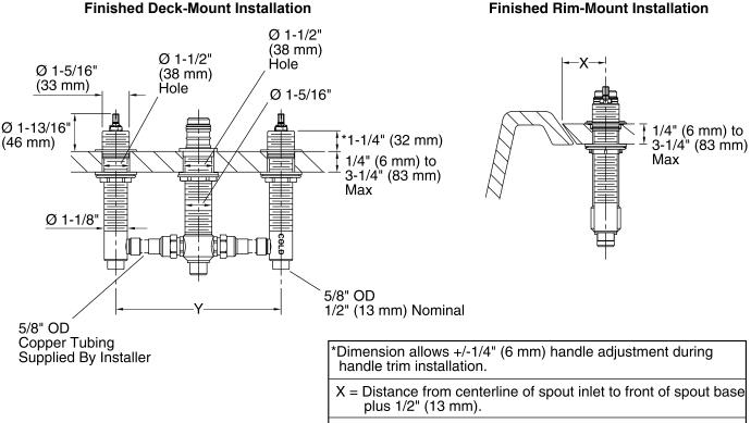
Y = Distance between valve body centerlines vary. Minimum distance is 8" (203 mm).
