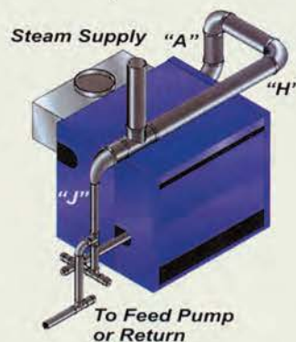
Recommended Minimum Pipe Sizes For Dual Risers
