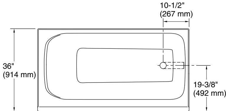
No change in measurements if connected with drain illustrated. (1381626)
