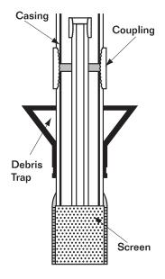
Debris Traps eliminate the common problem of loose dirt and stones plugging the pump suction area in water wells. The trap is quickly and easily installed over the well casing and secured with stainless steel clamp. Made of soft flexible PVC which conforms to irregularities of the drilled well. Does not crack or become brittle with age.
