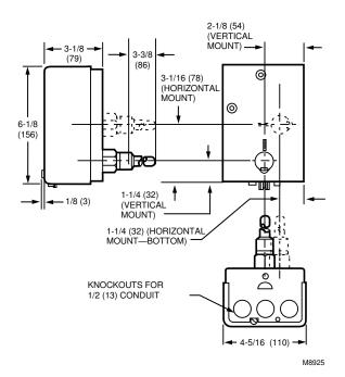
Fig. 1. L8148 dimensions in in. (mm).
