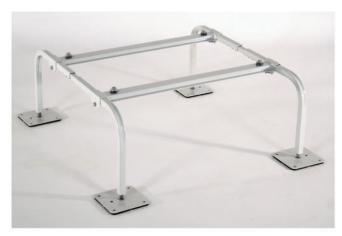
The Dual Fan Stand is made of 14-gauge square, steel tubing, and 11 gauge steel cross rails. This cuts down on vibration and enables the stand to hold up to 400 lbs.
