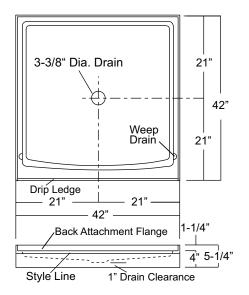
NOTE: Critical enclosure dimensions should be taken directly from the installed shower base with finished wall surround.
