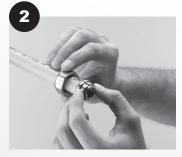
Slide nut over tubing, place retainer ring leaving one corrugation exposed.
