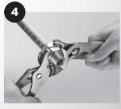
Tighten with wrenches until nut contacts body.
