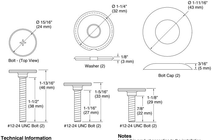
All product dimensions are nominal. Material: Steel, Plastic Install this product according to the installation guide.
