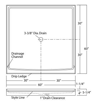
NOTE: Critical enclosure dimensions should be taken directly from the installed shower base with finished wall surround.
