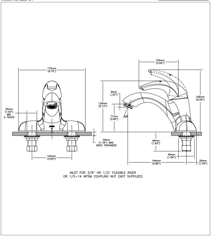
Delta reserves the right (1) to make changes to specifications and materials, and (2) to change or discontinue models, both without notice or obligation. Dimensions are for reference. Measurement may vary plus or minus 6mm(0.25"). Mounting locations are suggested only. Check with local codes for requirements in your area. This spec was produced July 24, 2018.
