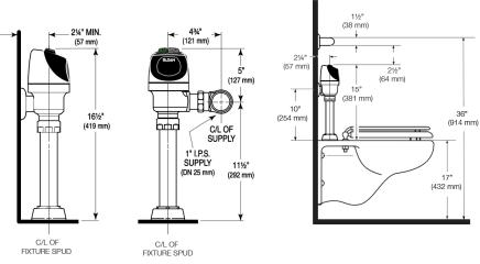
WHEN INSTALLING IN A HANDICAP STALL: Per the ADA Guildlines (section 604.9.4) it is recommended that the grab bars be split or shifted to the wide side of the stall. If grab bars must be present over the valve, use the alternate ADA installation as shown to the right.
