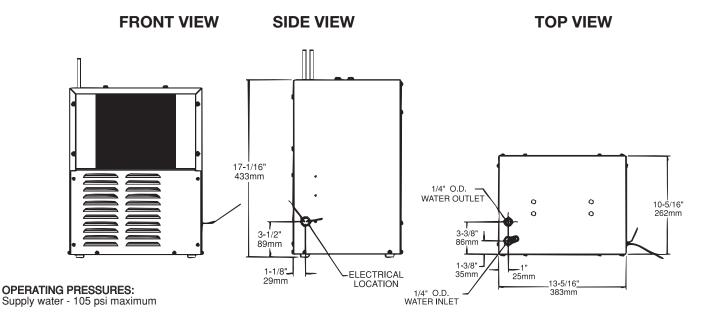
NOTE: A service supply stop (not included) should be installed at the cooler inlet line.
