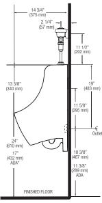
NOTE: All vitreous china dimensions shown in these drawings are nominal. Dimensions can vary within the tolerances established in the governing ASME A112.19.2/CSA B45.1 standard. Please take this into consideration when planning rough-in and plumbing layouts.
