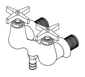
The leg tub fitting has a cast brass body with replaceable seats. The fitting body and spout are polished and chrome plated. The outlet spout is designed for a push on hose connection. The spout fits hose with a 1/2-inch inside diameter. The Quick-Pression quarter-turn compression stems are all brass with a double O-Ring seal and rubber seat washer. The handles are zinc die cast with a chrome plated finish.
