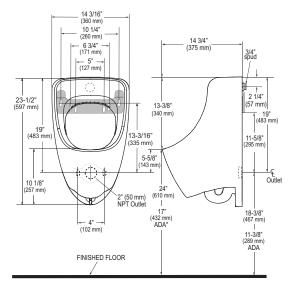
NOTE: All vitreous china dimensions shown in these drawings are nominal. Dimensions can vary wihin the tolerances established in the governing ASME A112.19.2/CSA B45.1 standard. Please take this into consideration when planning rough-in and plumbing layouts.
