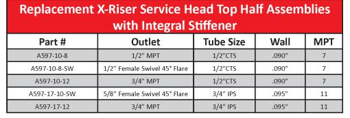
**Note:** The above part numbers are directly interchanchable with any X-Riser of the same corresponding tube size.
