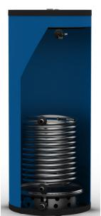
The tanks feature a high capacity stainless steel coil that efficiently transfers BTU's from the heat source to domestic water stored in the tank, making 1st hour delivery among the industry's best. Two-inch thick, high-density insulating foam with a tested R value of 13.4. surround the tank for low stand by losses. The SST series offer tank capacities 40, 65, 80 and 113 gallons to suit all your hot water needs.
