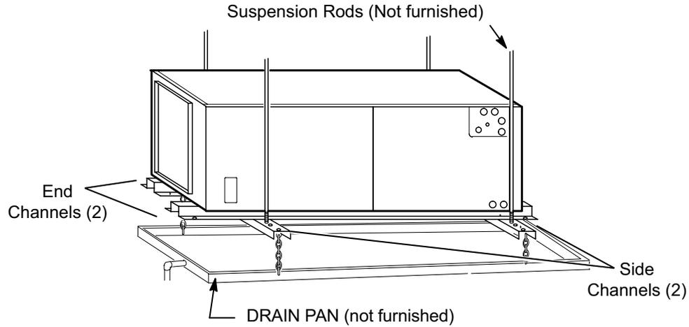
Includes (2) 1 x 1-1/2 x 32-5/8 in. side channels and (2) 1 x 3 x 53-7/8 in. end channels.
