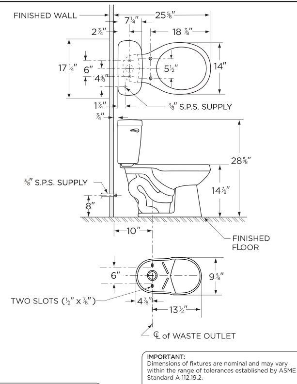
THIS FIXTURE QUALIFIES ACCORDING TO ASME TEST PROCEDURES AS A HIGH-EFFICIENCY WATER CLOSET WITH AN AVERAGE CONSUMPTION OF 1.28 gpf (4.8 Lpf) OR LESS.
