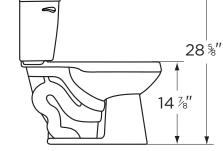
THIS FIXTURE QUALIFIES ACCORDING TO ASME TEST PROCEDURES AS A HIGH-EFFICIENCY WATER CLOSET WITH AN AVERAGE CONSUMPTION OF 1.28 gpf (4.8 Lpf) OR LESS.
