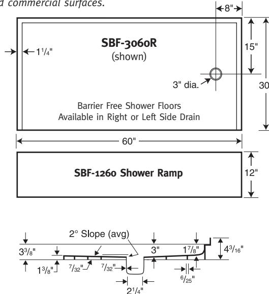
**IMPORTANT:** Rough-in dimensions are provided for reference only. You must measure the actual shower floor and check local building code requirements before construction of the stud wall. Meets ADA requirements for use in existing bathing facilities but not for new construction.
