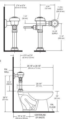
**NOTE**: All vitreous china dimensions shown in these drawings are nominal. Dimensions can vary within the tolerances established in the governing ASME A112.19.2/CSA B45.1 standard. Please take this into consideration when planning rough-in and plumbing layouts.
