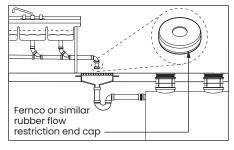
installing a valve or flow restriction cap on the sink piping that discharges into the drain. See drawing for guidance.
