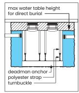
water. Great Basin™ models that are direct buried in high water table scenarios must be installed with an anchor kit. Model GB-1000 uses model AK3 anchor kit for use with deadmen anchors.
