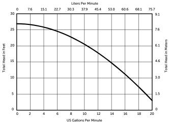
For proper performance, tank inflow cannot exceed pump discharge capacity at the installed head level. For technical assistance, consult the factory at 1-800-543-2550.
