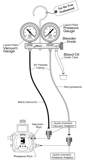
\*Can also be used on older pumps that have the vacuum port on the side of the pump.
