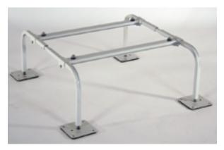
The Dual Fan Stand is made of 14-gauge square, steel tubing, and 11 gauge steel cross rails. This cuts down on vibration and enables the stand to hold up to 400 lbs.
