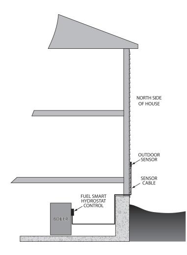
Before installation, determine the proper location for the sensor
