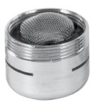
SLOTTED PART THREADS GPM NUMBER 2103 Female 55/64" - 27 2.2 2105 Dual 15/16 - 55/64" - 27 2.2 SLOTTED WATER SAVER
