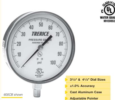
The 600CB Trerice Contractor Gauge is among the most frequently specified HVACR gauges within the construction industry. This gauge offers high reliability at a moderate price. The 600CB is furnished with a cast aluminum case and an adjustable pointer. Wetted parts are Lead-Free (PBF) brass.
