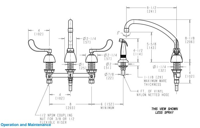
Installation should be in accordance with local plumbing codes. Flush all pipes thoroughly before installation. After installation, remove spout outlet or flow control and flush faucet thoroughly to clear any debris. Care should be taken when cleaning the product. Do not use abrasive cleaners,
