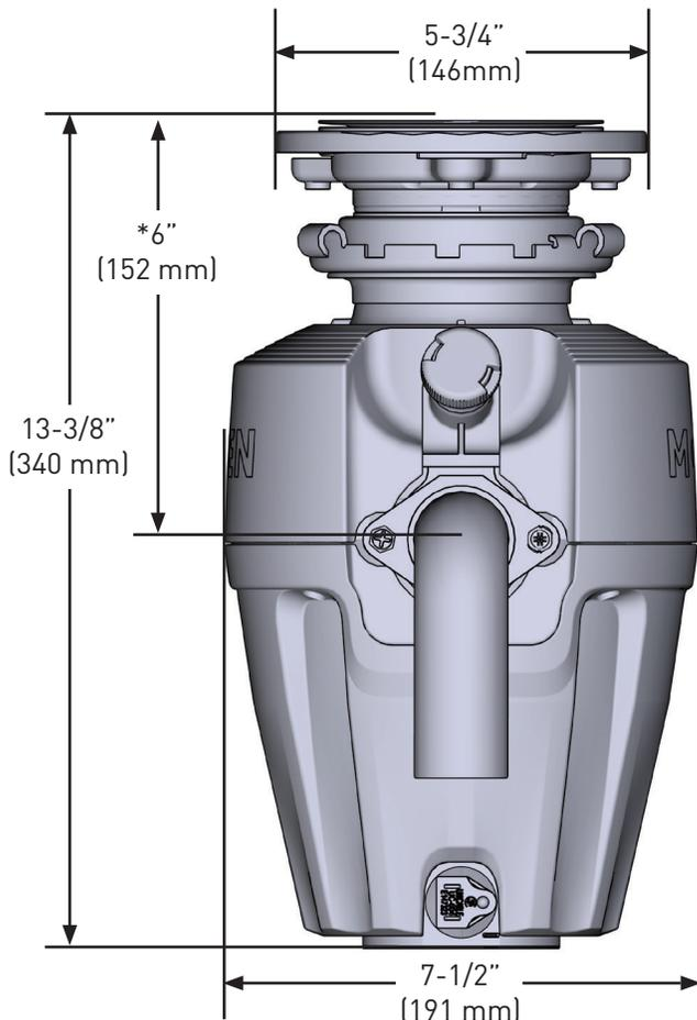
\*NOTE: Distance from bottom of the sink to center line of disposal discharge. Add 1/2" (13 mm) when a stainless steel sink is used.
