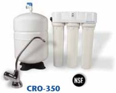
The CRO-350 is a 50\* GPD membrane R.O. utilizing a 3-stage filter system with a storage tank. Features high flowing Thin Film Composite (TFC) membrane. Easy to change filters and two gallon RO holding tank. A complete unit that is easy to install and is a more economical alternative.
