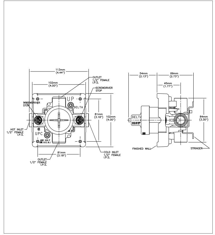
Delta reserves the right (1) to make changes to specifications and materials, and (2) to change or discontinue models, both without notice or obligation. Dimensions are for reference. Measurement may vary plus or minus 6mm(0.25"). Mounting locations are suggested only. Check with local codes for requirements in your area. This spec was produced May 24, 2015.
