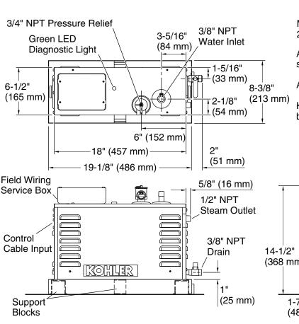
Minimum required access panel is 24" (610 mm) L x 15" (381 mm) H.
